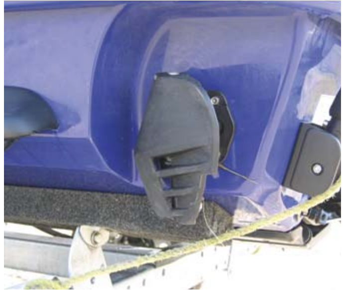
Figure 5: Bombardier Off-Throttle Control Flaps
