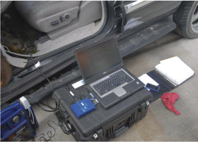
Figure 2: A laptop with translation software is connected to the vehicle's data port.
