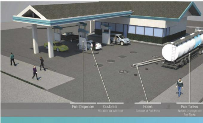
Figure 1. Typical gas station above ground view
