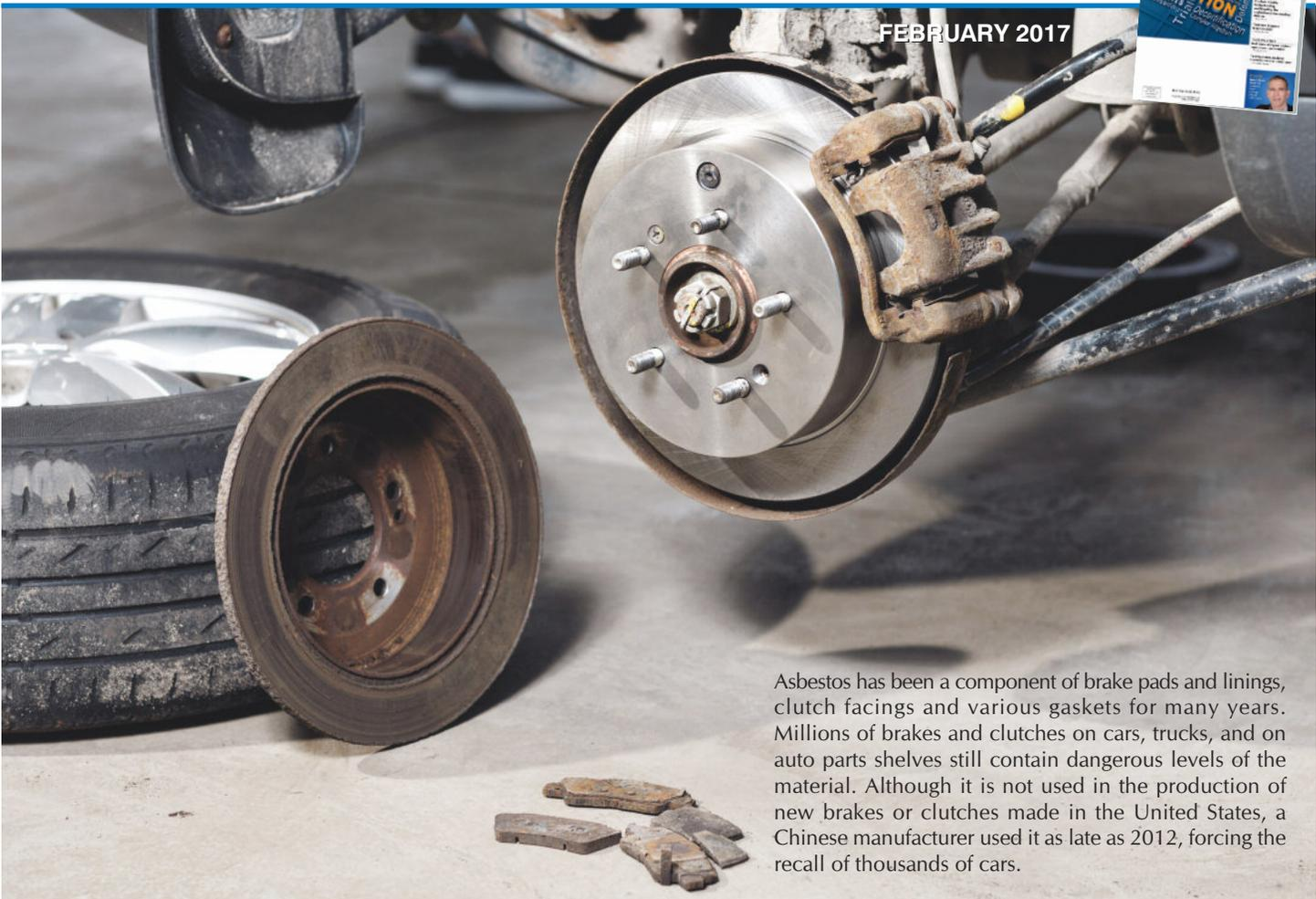
Asbestos has been a component of brake pads and linings, clutch facings and various gaskets for many years. Millions of brakes and clutches on cars, trucks, and on auto parts shelves still contain dangerous levels of the material. Although it is not used in the production of new brakes or clutches made in the United States, a Chinese manufacturer used it as late as 2012, forcing the recall of thousands of cars.
